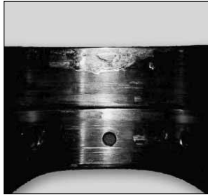
Figure 1. The inside surface of the bearing material is shown here, where it can be seen that the copper-lead overlay material has separated in certain areas.
