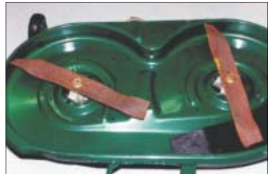
Figure 1: Severely corroded mower blades
